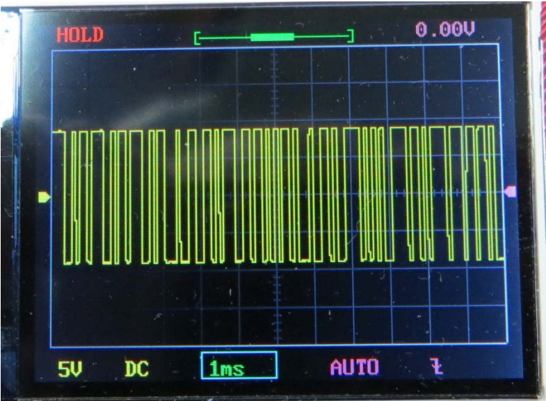
DSO DISPLAY SHOWING RS-232C OUTPUT SIGNAL FROM GARMIN (NOTE THE + AND - LOGIC LEVELS, APPROX +/- 9v )
